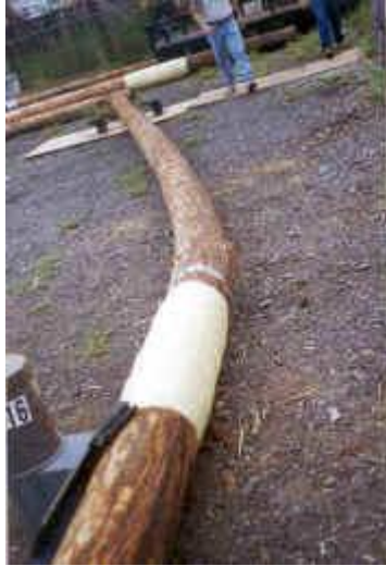
Pole Bent to Test Strength
